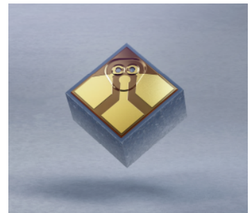
Chip die – two 850 nm VCSELs with single integrated photodiode for high-volume self-mixing interferometry sensing applications and integrated speed sensors
